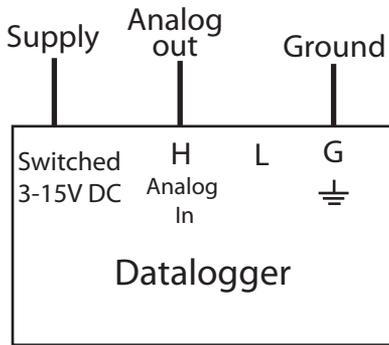
*Note: The acceptable range of excitation voltages is from 3-15VDC. If you wish to read the 10HS with Campbell Scientific data loggers, you will need to power the sensors off of the switched 12V port rather than the excitation port.*
